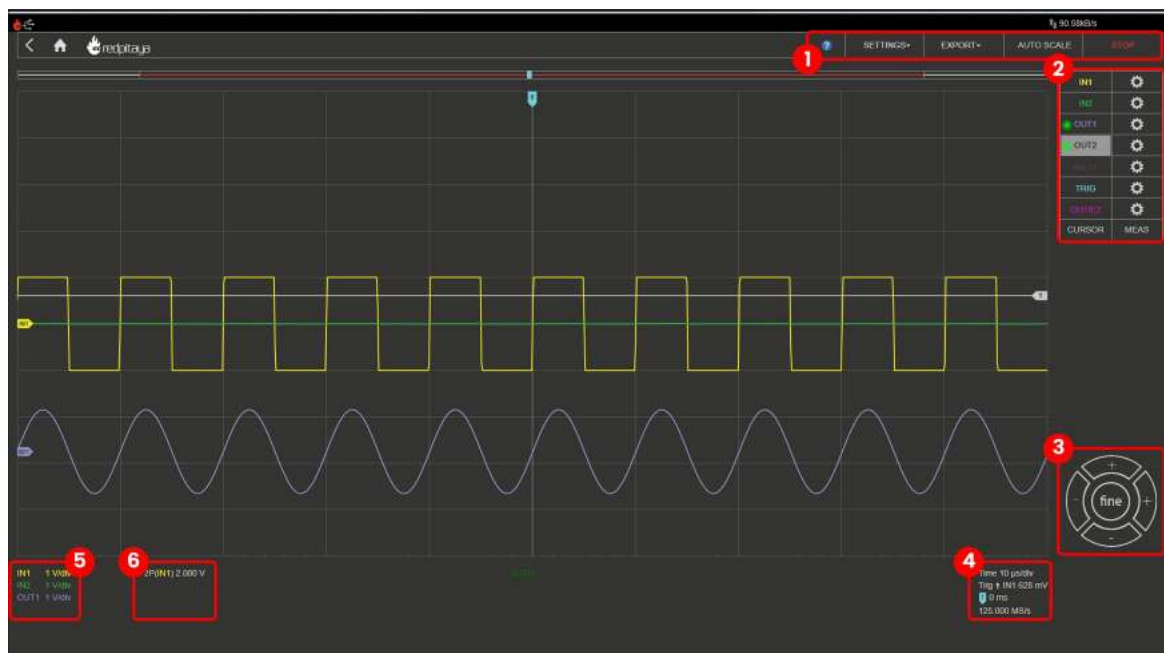
Figure 1.2: GUI of the Oscilloscope & Signal generator with pre-configured signal forms (Figure is taken from [DocSW])
