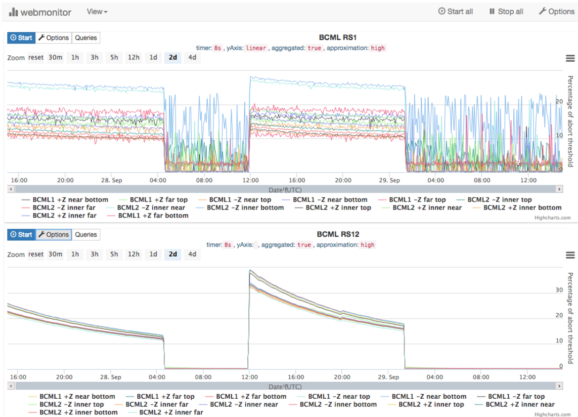
Figure A.12: The BCML web monitor displays the abort level in percent for RS1 and RS12. Two LHC fills can be seen with a duration of around 14 hours.
