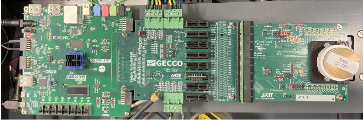
**Figure 3.4.: Single Chip Measurement Setup of the ATLASpix3** – From left to right: (1) FPGA: Nexys Video Board, (2) GECCO board, (3) Single Chip during a  $^{90}\text{Sr}$  measurement.
