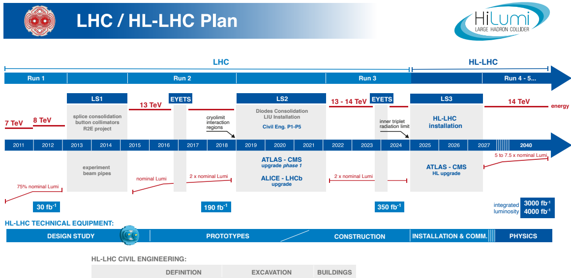
Figure 3.1: The High Luminosity LHC Upgrade schedule in November 2021. After passing two Long Shutdowns (LS1, LS2) and an Extended Year-End Technical Stop (EYETS) the LHC will enter Run 3 in 2022. Already during Run 2, the LHC doubled its nominal instantaneous luminosity. During the next operation period it is planned to increase the maximum center of mass energy to 14 TeV. During Long Shutdown 3 (LS3) the accelerator and experiments will undergo an extensive upgrade before entering the high-luminosity operation in 2027. [CER21b]
