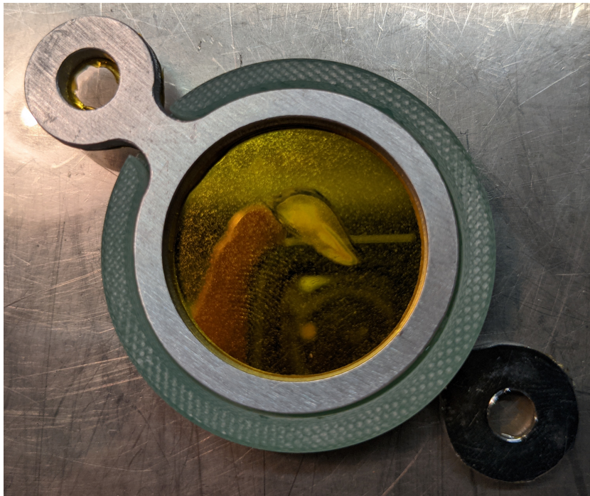
Figure 10.12.: Visual inspection of the 3 mm chamber after the long term measurement. A deteriorated spot on one electrode is visible. It compromised the charge collection efficiency of the chamber significantly.
