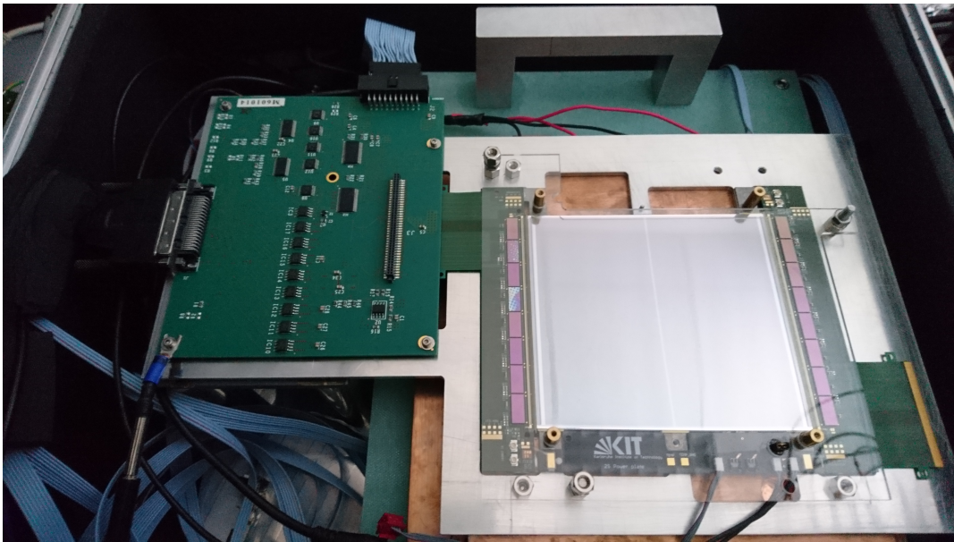
Figure 4.15.: Second functional 2S module built at KIT. A substitution for the SEH, a plate containing the high voltage filter circuit having the same dimensions as a SEH was used. On the image the module rests in its carrier and is placed inside the module readout station.
