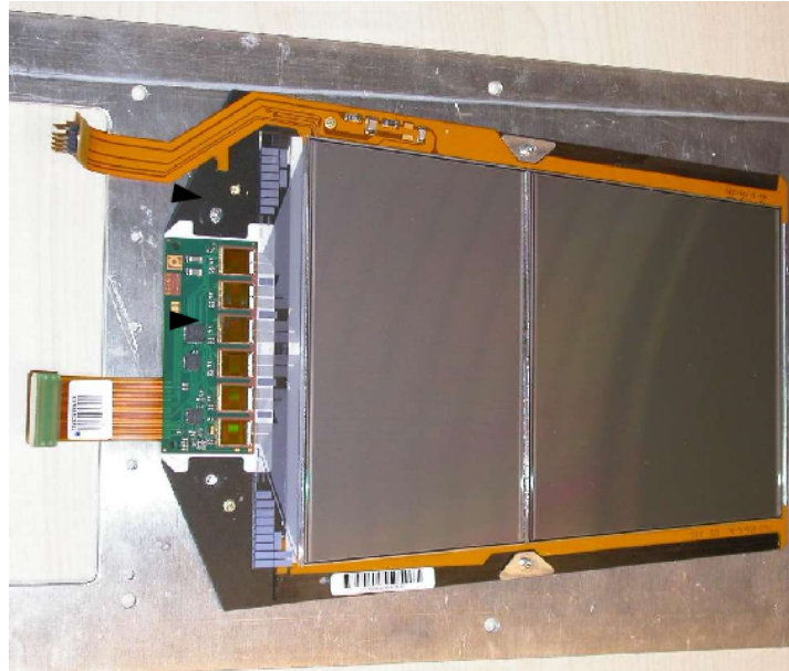
Figure 1.7. A CMS Silicon Strip Tracker module and its hybrid (green). A row of six APV25 chips can be seen wire-bonded to the strips [30].
