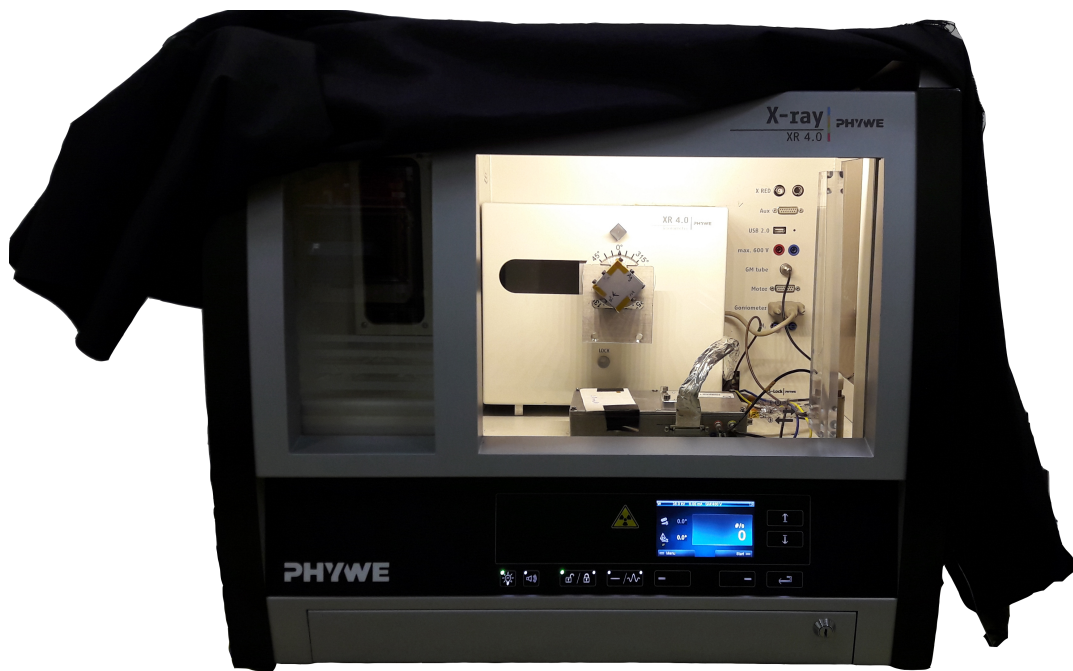
Figure 2.2. The Phywe XR 4.0 Expert Unit with X-ray light source used for the threshold calibrations.
