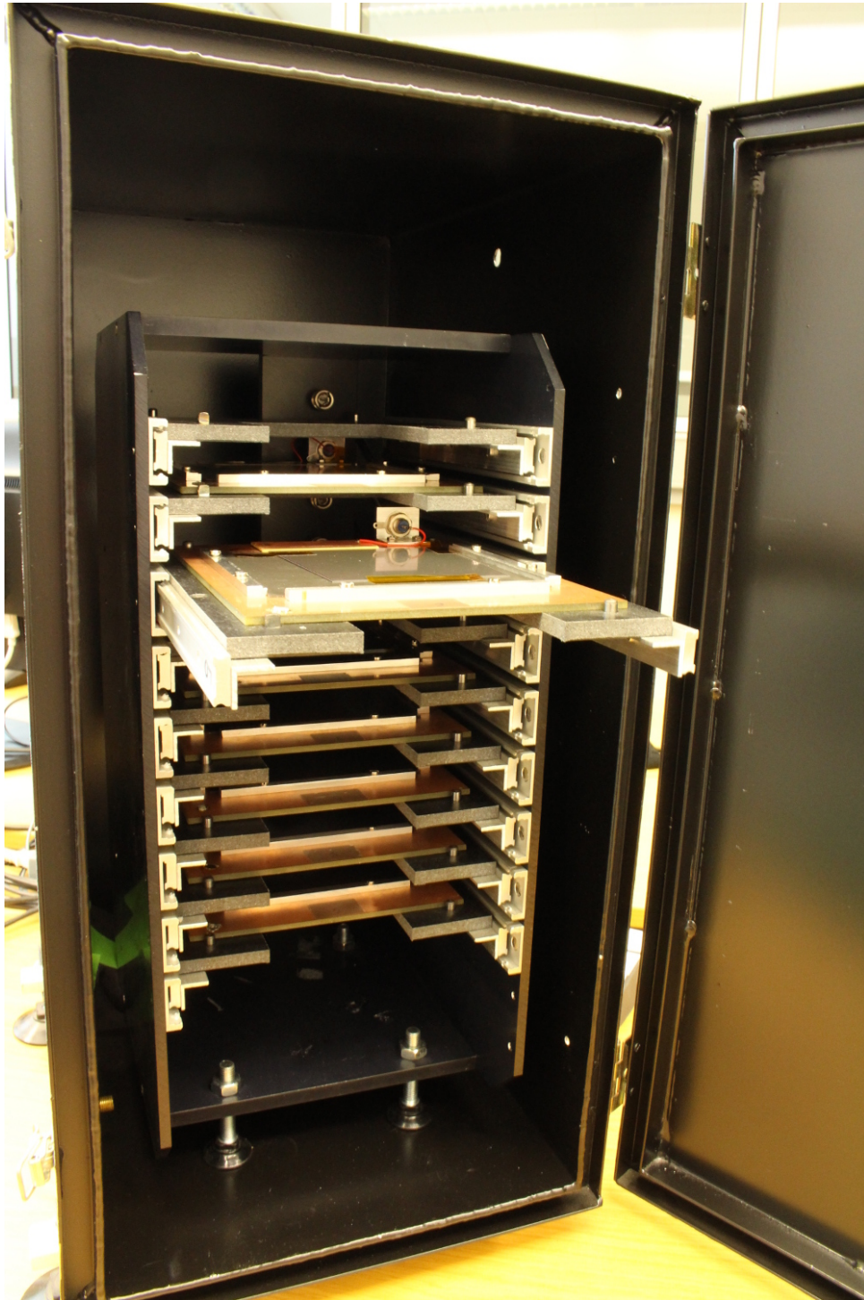
Figure B.1.: Sensor rack used in the sensor long-term station with ten telescopically mounted layers onto which the copper plates with the silicon sensors can be mounted. The rack provides a set of sockets at its back side which corresponds to the plugs on the sensors' copper plates. By sliding each layer into the rack, the plugs are connected with the corresponding sockets and the bias voltage and ground connection are applied to the sensors.
