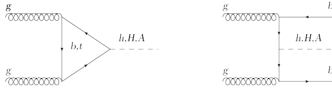
Figure 1.3: The two dominant production modes for neutral heavy Higgs bosons: Production via gluon fusion (left) and b-associated production (right).
