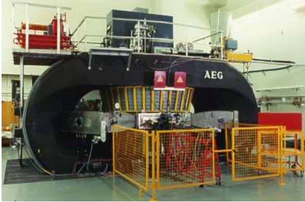
Figure 3.3: Picture of the isochron cyclotron at the Forschungszentrum Karlsruhe
