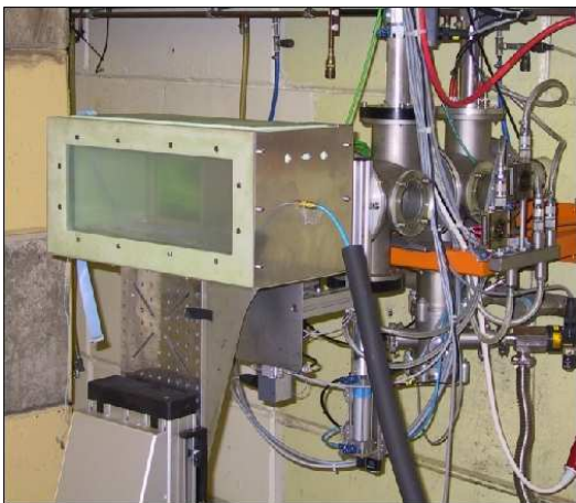
(a) Insulated box on the X-Z-stage. The beam pipe can be seen on the right.
